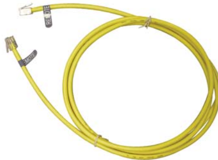
Figure 3-24, REMOTE Communication Cable (300V)
