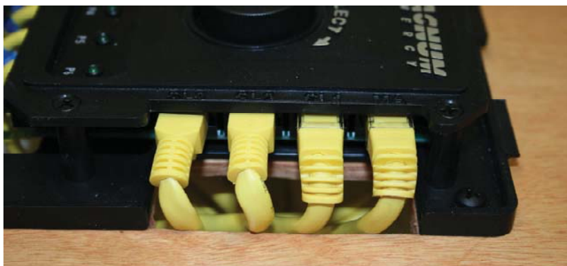
Figure 2-6, Connecting the CAT 5 Cables to the Router
