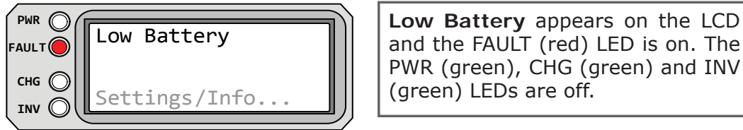
Figure 5-18, Low Battery Fault
